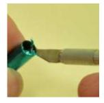
Step 5A & B: Remove any excess foil from the ends of the tube with either a small pair of scissors or use an exacto knife to trim the ends flush with the end of the tube. You are doing this so when you plug the ends of the tube, you will obtain a tight seal on the tube.
