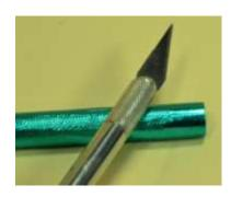
Step 6: Use the end of the Exacto knife to "texture" the foil to hide the seam and to make the blank more visual pleasing.
